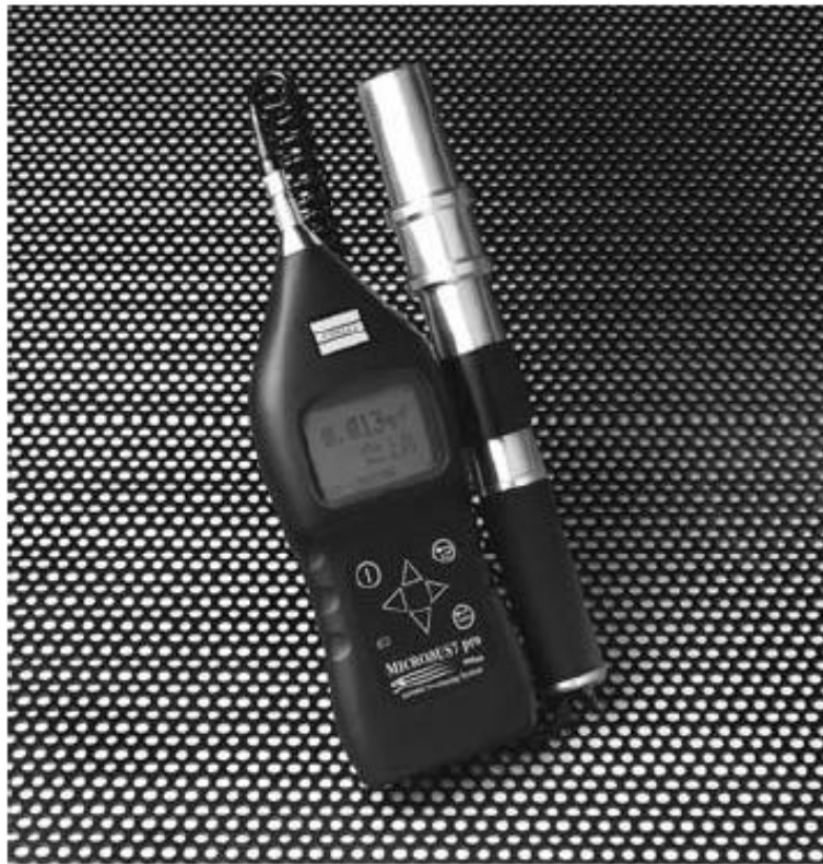
Figure 14.4. Casella Microdust-pro™ measures the concentration of suspended particulate matter with a range of 0.001 mg/m 3 to 2500 mg/m 3 . (Courtesy of Casella USA.)
