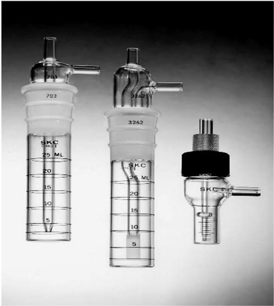
Figure 6.4. Examples of liquid-filled collection devices. Left to right: a midget impinger, a midget bubbler, and a spill-proof impinger. (Courtesy of SKC, Inc.)
