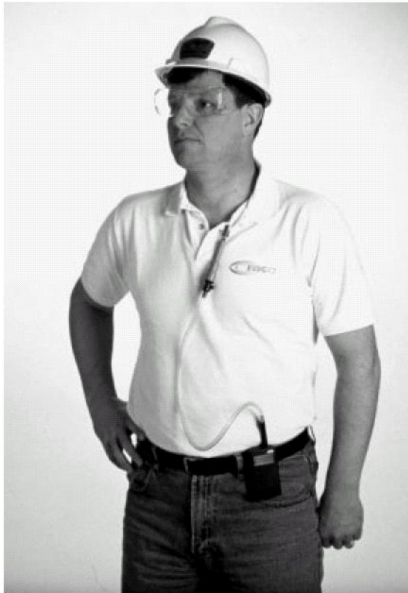
Sorbent tube placement with protective tube holder
