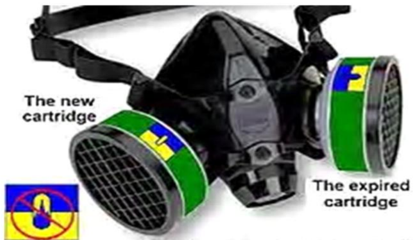
The North respirator 7700 with cartridges RT 41 (ammonia) with ESLI. The indicator is in the field of view of the employee (oval window in the center changes color after saturation of the sorbent)
