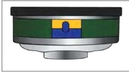
Figure 3—The yellow is completely gone when the service life of the cartridge is expired.
